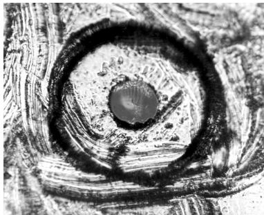
Figure 7-7. Damage from improper cleaning
