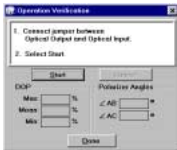
Figure 6-21. Operation Verification window
